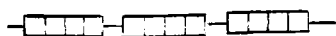
C Stepladder polymer. A hybrid of conjugated ladder and conjugated linear structures.
